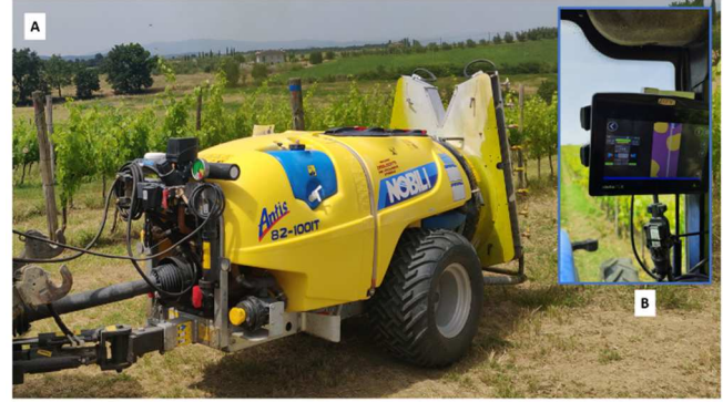
Fig. 3. (A) Variable rate sprayer Nobili model Antis (B) detail of the virtual terminal with prescription maps.
